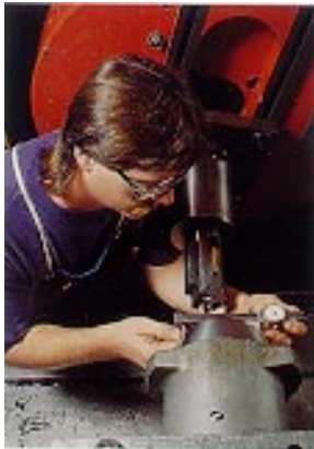
Manufacturing accuracy is maintained to within +/- 0.001" of the dimensions specified.
