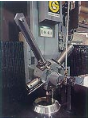
Valve bodies are cut to precision tolerances by a computer-controlled vertical turret lathe.
